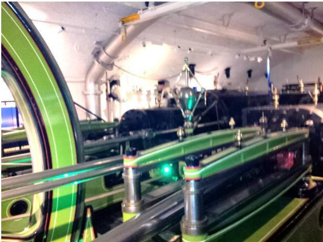
The picture above shows the original steam engine hydraulic pump
