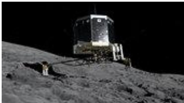
Once a suitable landing site was chosen, the lander was released from a height of about one kilometre. Touchdown took place at walking speed — less than one metre per second. Unfortunately it bounced and drifted across the comet before finally coming to rest in the shadow of a mountain. This deprived it of the power needed for a complete analysis of the surface via the installed experiments but nevertheless much valuable information was gained before the batteries were finally exhausted.
