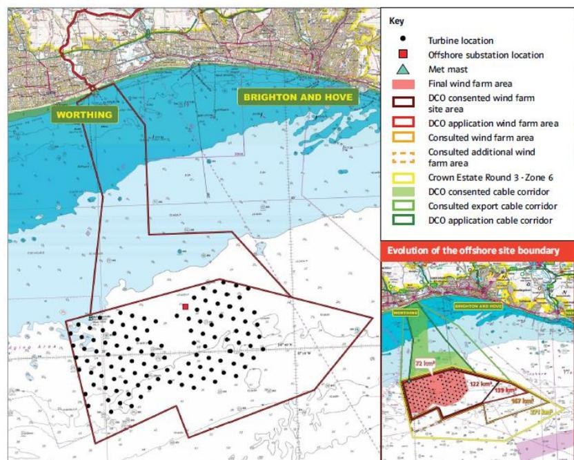
**Undersea Supply** VBMS, a Netherlands company that specialises in subsea power cable installation will be responsible for the installation (lay and simultaneous bury) at a depth of 1.5 to 2.0m two 16 kilometre-long, 3 core aluminium, 150kV High Voltage Alternating Current (HVAC) export cables from the offshore substation to the onshore cable junction at Brooklands Pleasure Park using the DP2 cable-laying vessel *Stemat Spirit*.
