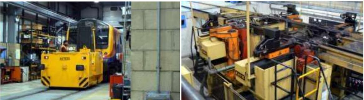
**Reprofiling lathe with train about to be towed in place**
