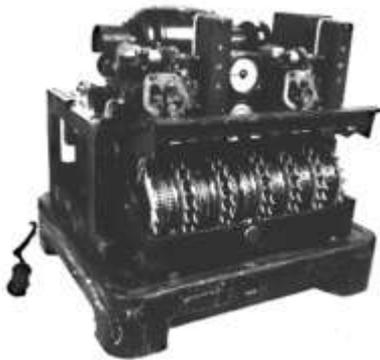
*The Lorenz was an even more complex cipher machine than Enigma. Made by the Lorenz company, it was used exclusively for the most important messages passed between the German Army Field marshals and their Central High Command in Berlin. Its size meant that it was not a portable device like Enigma. Bletchley Park code breakers called the machine 'Tunny' and the coded messages 'Fish'.*
