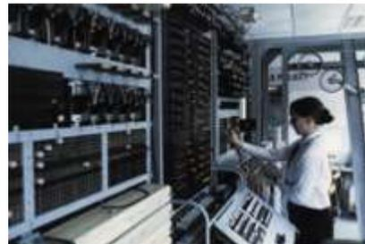
*analyses on the intercepted messages. Colossus could read paper tape at 5,000 characters per second and the paper tape in its wheels travelled at 30 miles per hour. This meant that the huge amount of mathematical work that needed to be done could be carried out in hours, rather than weeks.*
